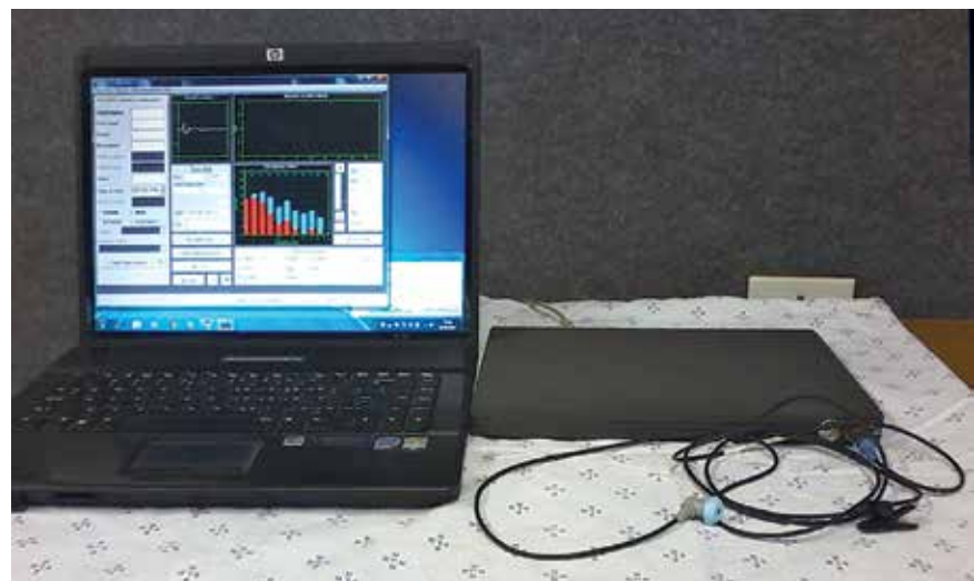
DP Echoport ILO 292 connected to PC, used for DPOAE testing
