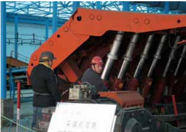
A miner being trained at a surface facility on an underground longwall shearer cutting machine, with powered roof supports in the background, at a coal mine in Shandong Province, China
